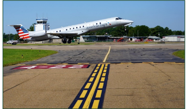
Holding Position for Runway 4-22 at Taxiway C
